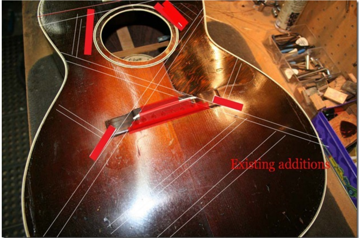
Additions by previous repairs
