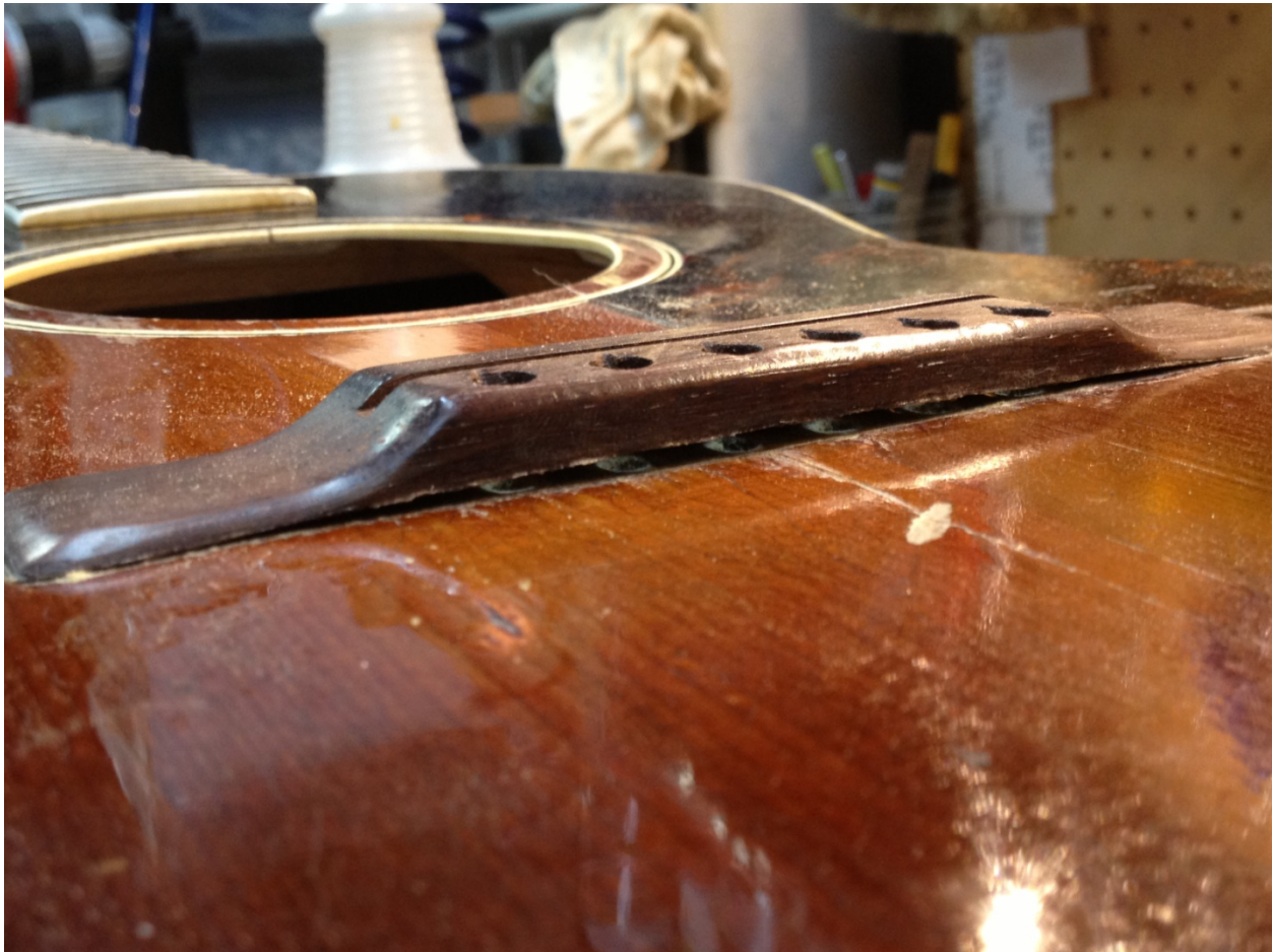
Original rosewood bridge distorted by previous bulge along transverse axis, resting on repaired top. Previous bulge along longitudinal axis was much greater.
