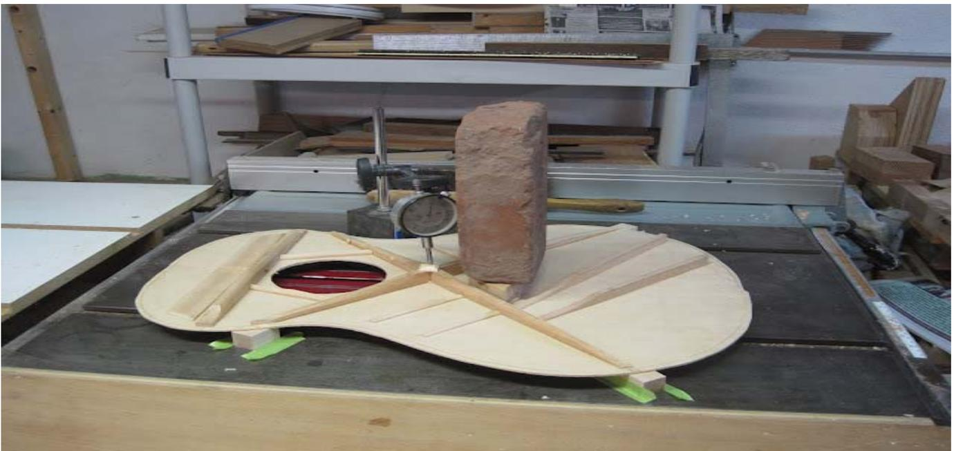
After I get this to behave the way I want it to I have one last thing to do. I tune the tone bars by ear, tapping, listening and shaving. This is the only subjective part of the whole process and all I am looking to do is achieve a balanced and fairly dead sound from the lower portion of the soundboard. While tapping at the bridge area on the top. Then I am ready to build the box.
